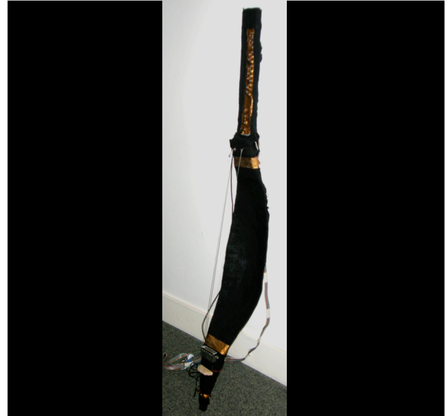
The Convolin prototype was hand-built out of a wire frame coated with fiberglass.
